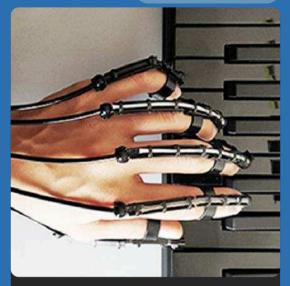
When gas or hydraulic pressure is applied, the length of the contracting (stretching) muscle fibers shortens (elongates), generating linear force in the direction of tension.
