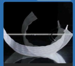
The membrane is welded into a specific pattern to form a membrane-like airbag. When the airbag inflates, the internal pressure increases, causing the airbag to bulge and drive the membrane to deform.
