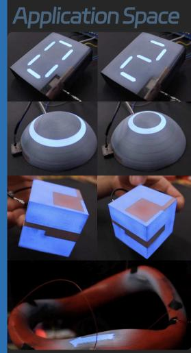
Electroluminescent materials can emit light when driven by 100-200V DC or AC power. A single luminescent material typically emits only one fixed color.
