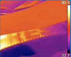
By flowing liquids of different temperatures through fine channels beneath the surface of an object, the surface temperature of the material can be dynamically altered.
