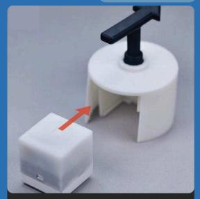
With several small robots capable of translation and rotation, along with various modular shells, different movement modes and interactive functions can be achieved.
