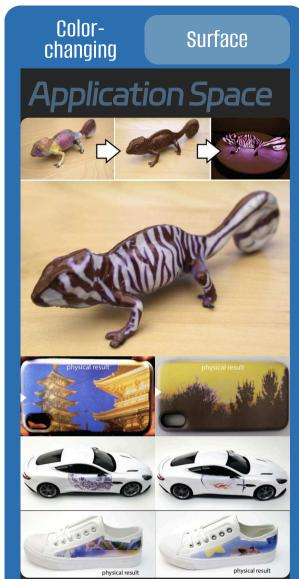
Upon UV exposure, the pigment turns black; under different visible light exposures, the pigment can change to other colors. The coloration time of the pigment depends on the intensity of the exposure source, typically requiring 1-10 minutes. The natural fading time of the pigment is influenced by the ambient light intensity, usually taking 5-24 hours. The pigment has a limited color range, with green being particularly lacking in the coloration spectrum.
