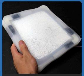
When the material is inflated, it softens, and the structural shape can be changed through the length adjustment of the telescopic rods. When the material is vacuumed, it hardens, and the altered shape remains fixed.
