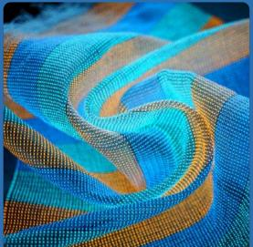
When conductive weft yarns and luminous warp yarn fibers are woven with cotton yarn, each interwoven warp and weft forms an EL unit, which emits light when an alternating voltage is applied.
