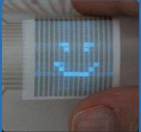
A thin-film electroluminescent display consists of two overlapping electrodes. When an alternating signal is applied, the electroluminescent coating between the electrodes lights up, causing the display to emit light.
