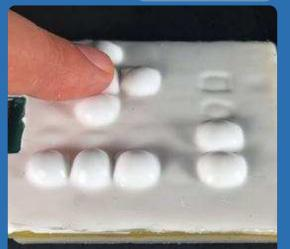
Each deformation pixel consists of an electroosmotic pump. When an electric field is applied, the liquid inside the pixel flows upward, causing the top membrane layer to undergo bulging or indentation deformation.
