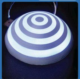
By spraying electrodes and luminescent materials onto the surface of an object, a display can be achieved on any shaped surface when an alternating electric field is applied.
