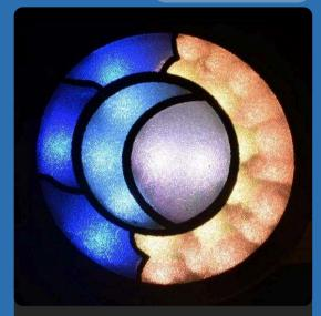
Use reflective materials and lightdiffusing fillers to design the distribution of LED light in threedimensional space.
