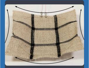
By selecting different shape memory alloys and custom-woven substrates, three basic deformations—bending, expansion, and contraction—can be achieved.
