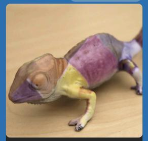
Photochromic pigments are sprayed on the surface of an object, and when exposed to different colors of light, the pigments change to different colors.
