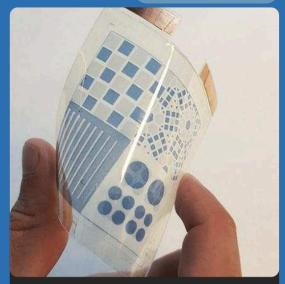
When a voltage is applied, the electrochromic material can change its color from nearly transparent to a deeper blue.
