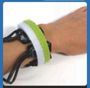
A Peltier element array can heat up or cool down when powered, thereby altering the surface temperature of the object.
